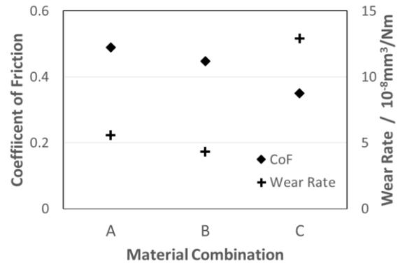
**Figure 1:** Mean coefficient of friction and pin wear rate for three pin / disk material combinations – (A) Zirconia / Alumina (B) Zirconia / ZTA (C) Ruby / ZTA.
