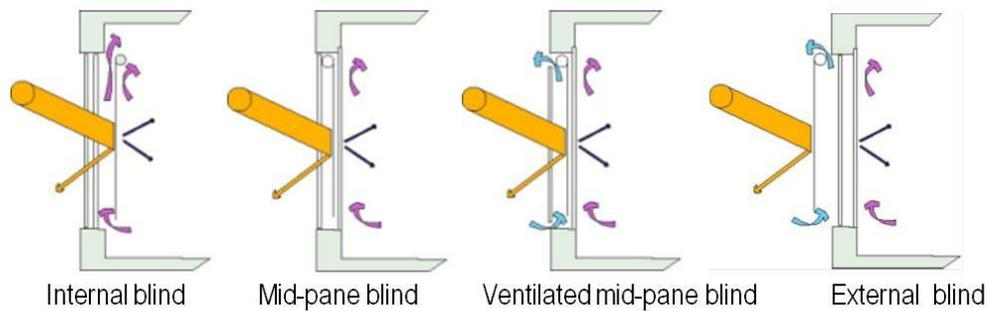
Figure 2. Range of layered glass facades incorporating shading.
