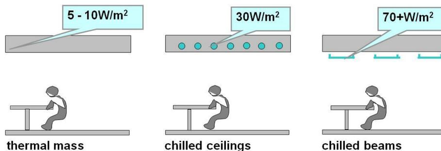
Figure 5. Chilled surface options: thermal mass (with night cooling), chilled ceiling and chilled beams.
