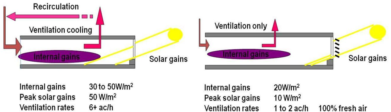
Figure 4: Comparison of a more traditional all-air ac system with a 'decoupled' chilled ceiling system, indicating the level of reduction in internal heat gains and solar heat gains, through the above design strategy, and not requiring any air recirculation.
