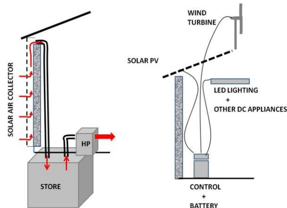
Figure 8. Example of building integrated energy supply and energy storage for a thermal system, using a TSC air collector, and an electrical system, combining solar PV and wind (SOLCER project, Wales Low Carbon Research Institute).
