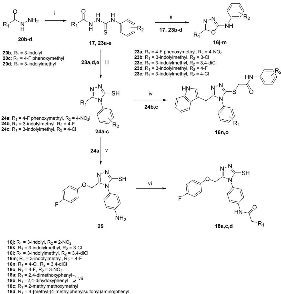
**Scheme 3.** Reagents and conditions: (i) substituted phenylisothiocyanate, ethanol, reflux, 1 hr; (ii) 1,3-dibromo-5,5-dimethylhydantoin, acetonitrile; (iii) a- NaOH or saturated Na<sub>2</sub>CO<sub>3</sub>, reflux, 3 hrs; b- HCl, H<sub>2</sub>O; (iv) phenylacetyl bromide, KOH, 70% ethanol, rt, 12 hrs; (v) Fe, HCl, ethanol, H<sub>2</sub>O, 90°C, 1 hr; (vi) R<sub>2</sub>COCl, THF, K<sub>2</sub>CO<sub>3</sub>, rt, 4 hrs; (vii) BBr<sub>3</sub>, DCM, 0°C, 2 hrs.
