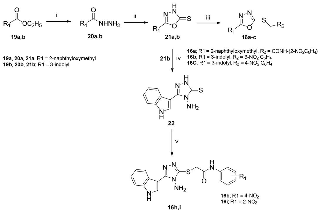
**Scheme 1.** Reagents and conditions: (i) N<sub>2</sub>H<sub>4</sub>·H<sub>2</sub>O, ethanol, 90°C, 1 hr; (ii) a- CS<sub>2</sub>, KOH, 80% methanol, 100°C, 12 hrs; b- H<sub>2</sub>O, HCl; (iii) alkylchloride, NaOH, H<sub>2</sub>O, ethanol, 90°C, 7 hrs; (iv) a- N<sub>2</sub>H<sub>4</sub>·H<sub>2</sub>O 80%, reflux, 2 hrs; b- H<sub>2</sub>O, AcOH; (v) nitrophenylchloroacetamide, NaOH, ethanol, H<sub>2</sub>O, rt, 5 hrs.
