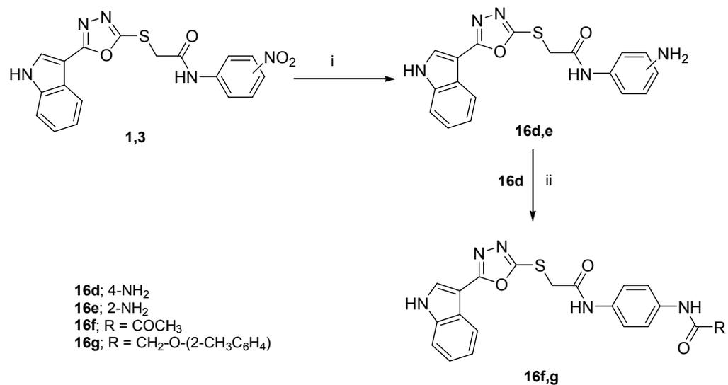
**Scheme 2.** Reagents and conditions: (i) Fe, HCl, ethanol, H<sub>2</sub>O, 100°C, 1 hr; (ii) RCOCl, THF, K<sub>2</sub>CO<sub>3</sub>, rt, 5 hrs
