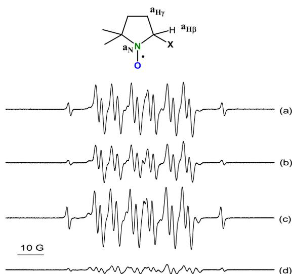
**Figure 3.** EPR spectra of DMPO spin adducts obtained during the decomposition of CHHP in cyclohexane in the presence of: (a) AgPd/MgO, (b) Pd/MgO, (c) Ag/MgO, and (d) autoxidation with no catalyst. All catalysts were prepared *via* sol immobilization.
