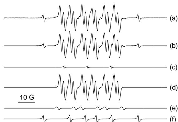
**Figure 4.** Deconvoluted EPR spectra of DMPO spin adducts obtained during the decomposition of CHHP in cyclohexane in the presence AgPd/MgO with a Ag:Pd molar ratio of 1:1. (a) experimental spectrum and b simulated spectrum, (b) simulated spectrum, (c) di-*tert*-butyl-nitroxide derivative, (d) DMPO-O-C<sub>6</sub>H<sub>11</sub> spin adduct, (e) DMPO-O<sub>2</sub>-C<sub>6</sub>H<sub>11</sub> adduct, and (f) carbon centred adduct, which is possibly a DMPO-C(OH)R<sub>2</sub> species.
