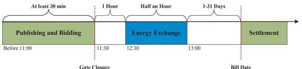
Fig. 3. An example of processing of an order in Elecbay.
