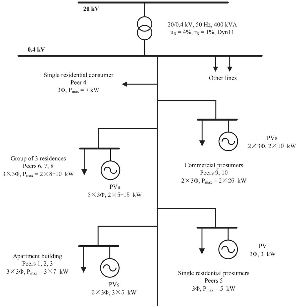
Fig. 6. The Benchmark LV Microgrid adapted from [29].
