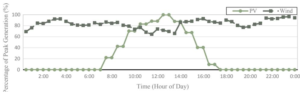
Fig. 9. PV and wind generation profiles in Case Study 5.2.
