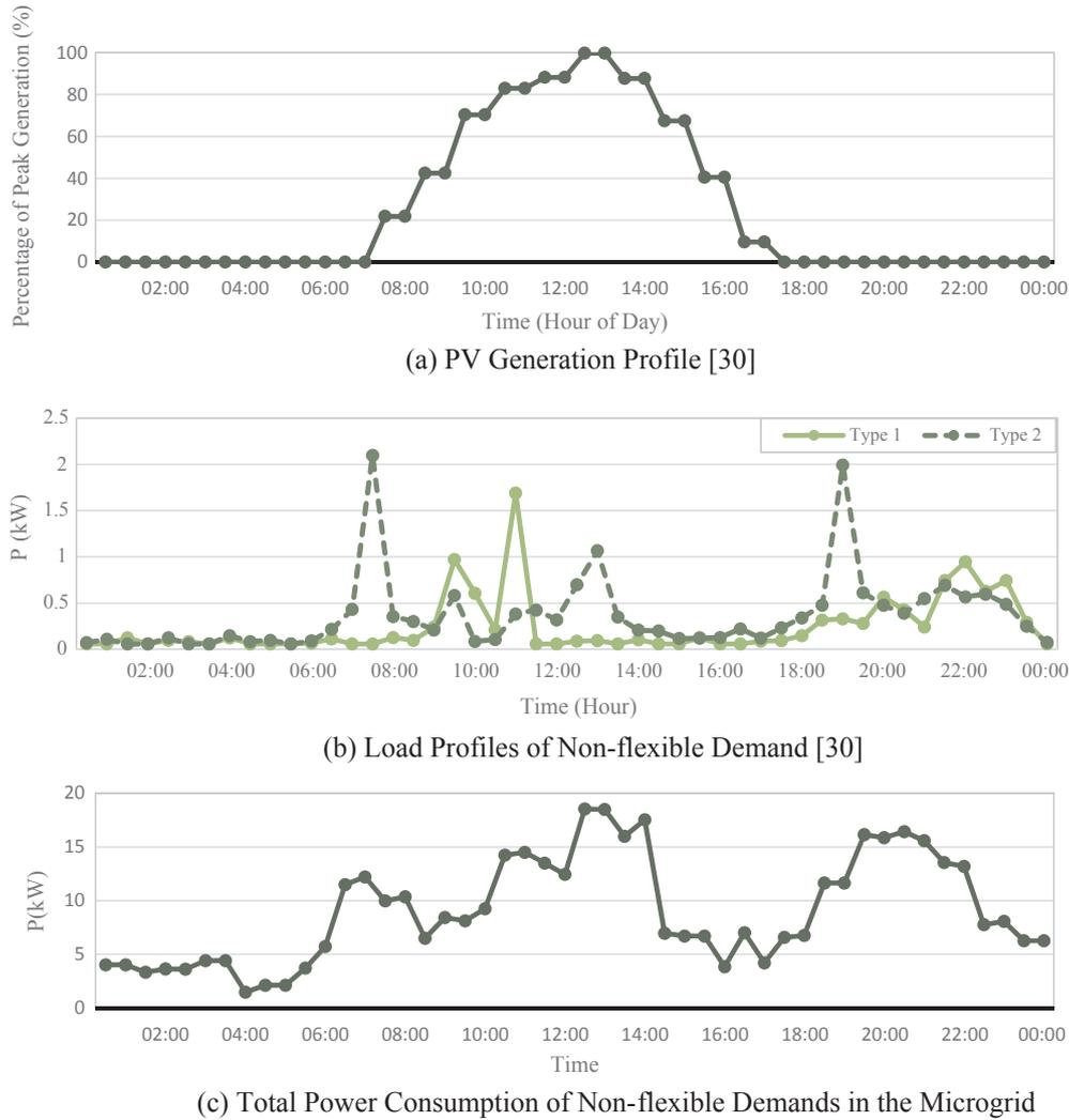
Fig. 7. Input data of Peers 1 and 2, and the total non-flexible demands of the Microgrid in Case Study 5.1.
