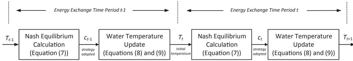
Fig. 5. The procedure of the multi-time period simulation.
