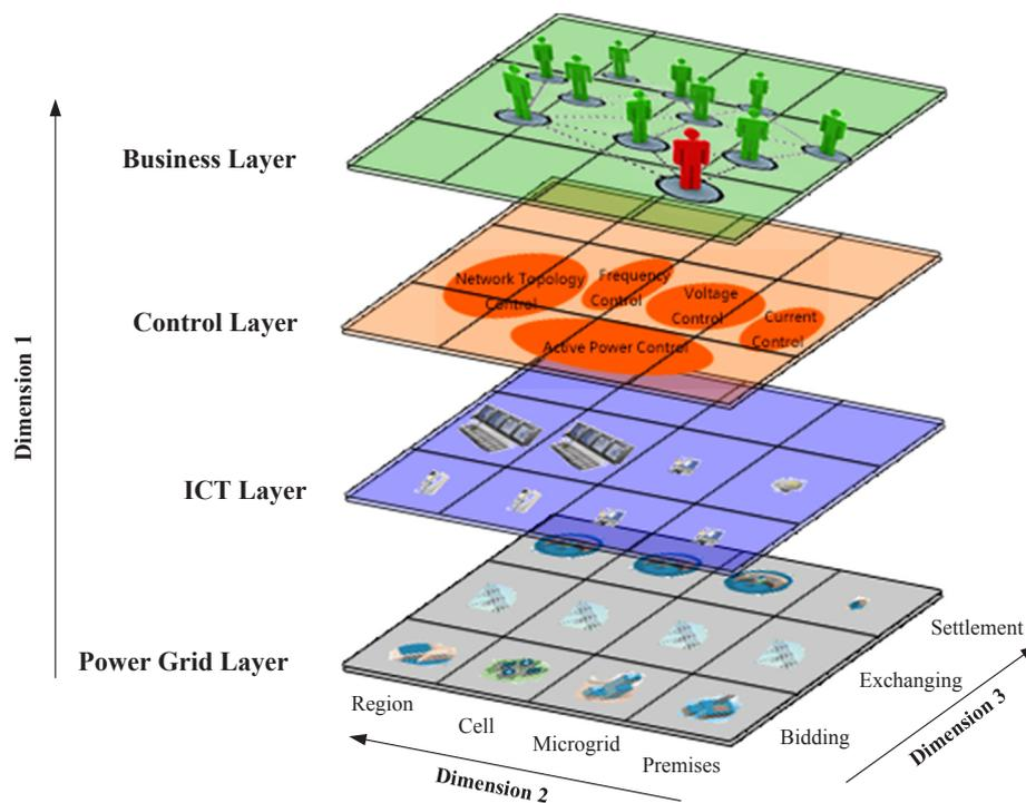
Fig. 1. A four-layer system architecture of Peer-to-Peer energy trading.
