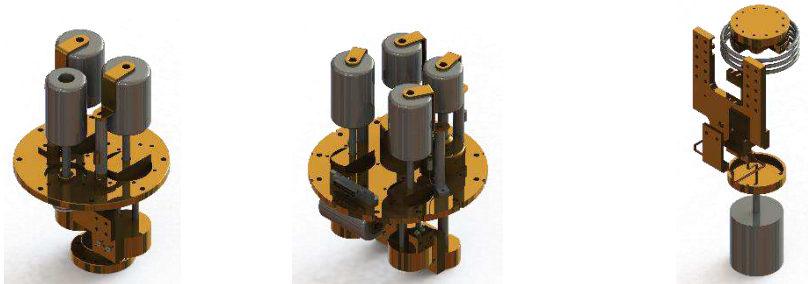
Fig. 4: The three closed cycle fridges to cool down from 4K to 100mK. Left to right: the 1K continuous operation fridge, the 350 mK for continuous operation and the 100 mK mini dilution fridge. All of them will be supplied from Chase Research Cryogenics, the first one has been delivered.
