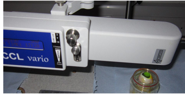
Figure 1. Laboratory set-up [authors own] for riboflavin/UVA corneal cross-linking of an enucleated porcine eye. Note the bright yellow fluorescence of the stromal riboflavin as the cornea is exposed to UVA light from above. UVA, ultraviolet.
