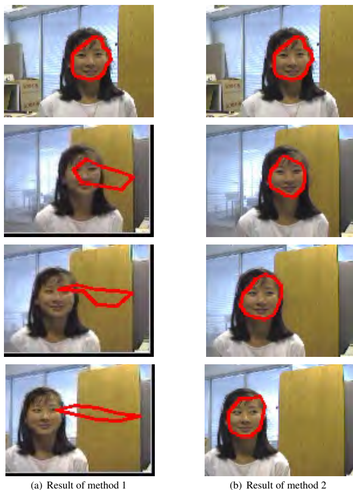
Fig. 6 Head sequence with fast motion. The red closed curve indicates the contour. From top to bottom are the frames with No.0, 18, 22 and 25. Column (a) is the result of method 1, (b) is the result of method 2 (our method).
