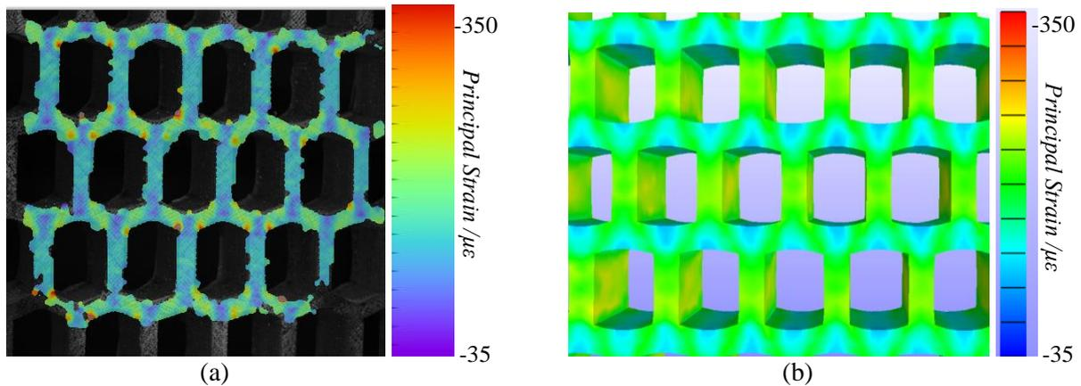
Figure 5. Example of (a) DIC and (b) FEM data for structure with staggered cells, with images showing results at 18% elongation in the vertical direction.
