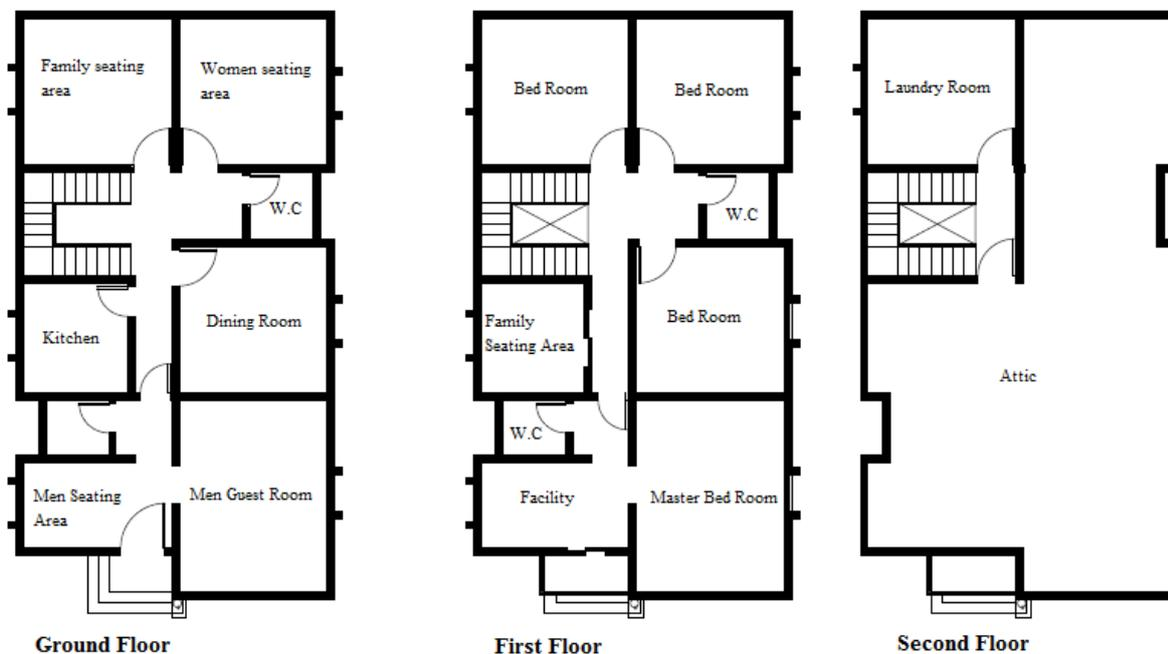
Fig 5.2- Layout Design of House Prototype2
