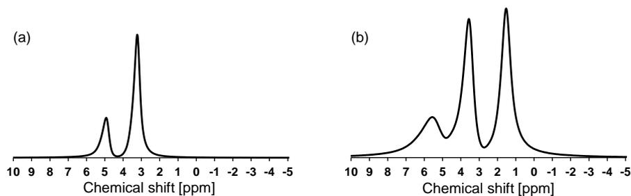
**Figure 2.**  $^1\text{H}$  NMR spectra of (a) methanol and (b) 1,4-butanediol in Pd/TiO<sub>2</sub> catalyst.
