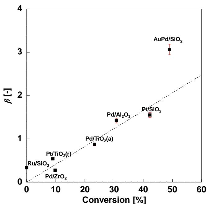
**Figure 45.** Plot of  $\beta$ , as defined in Equation (2) against catalytic conversion. Note that (a) indicates TiO<sub>2</sub> anatase and (r) indicates TiO<sub>2</sub> rutile. The dotted line is a guide to the eye.
