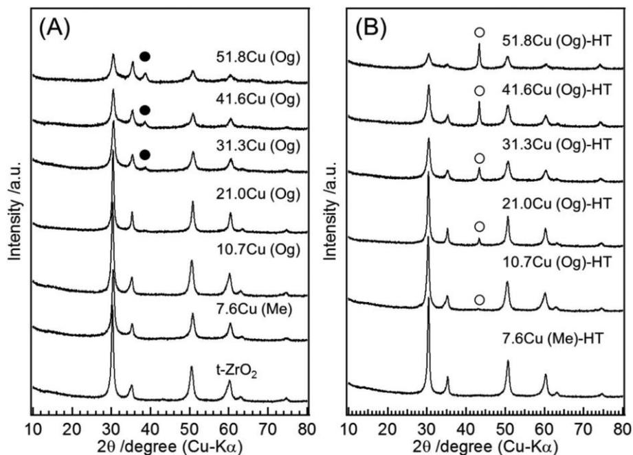
Fig. 2 PXRD patterns of (A) calcined catalysts, (B) reduced catalysts; ● CuO, ○ Cu metal. HT = heat treated.
