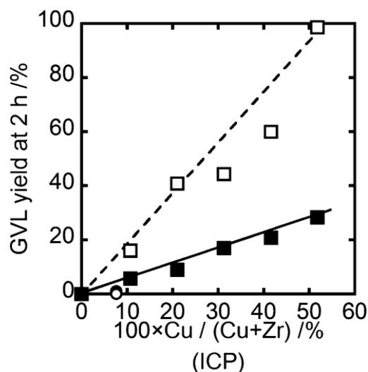
Fig. 1 GVL yield as a function of Cu/(Cu + Zr) ratio determined by ICP. ○ Me-HR, ● Me, ■ Og, □ Og-HR. Reaction conditions: 200 °C, 35 bar H<sub>2</sub>, 0.050 g catalyst, 5 wt% LA in water, 2 h.
