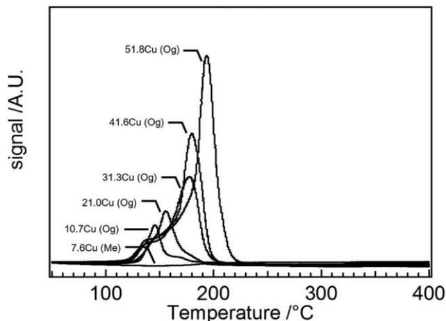
Fig. 3 TPR spectra of Cu–ZrO<sub>2</sub> catalysts after calcination.
