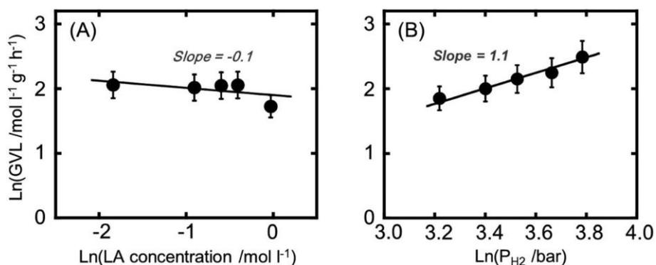
Fig. 6 Effects of concentration of LA (A) and hydrogen pressure (B) on the hydrogenation of LA over 51.8Cu(Og)-HR. Reaction temperature: 200 °C; 30 min; 25–60 bar H<sub>2</sub>, 0.010–0.050 g catalyst, 2.5–15 wt% LA in water.
