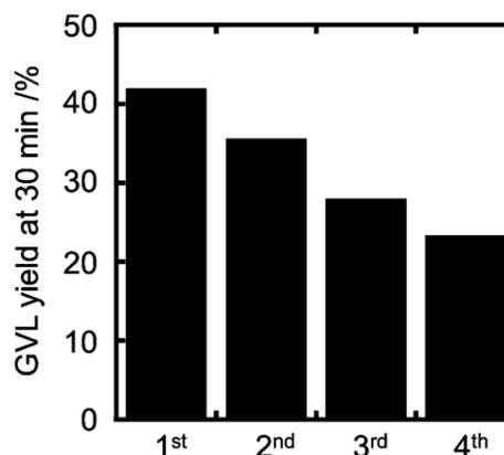
Fig. 7 Reusability data for 51.8Cu (Og)-HR catalyst. Reaction temperature: 200 °C; 30 min; 35 bar H<sub>2</sub>, 0.050 g catalyst, 5 wt% LA in water.
